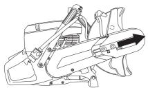
• Remove the belt from the belt pulley.
